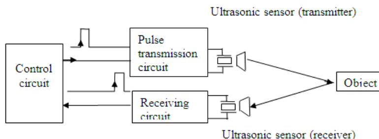
Fig: Block diagram of ultrasonic sensor
