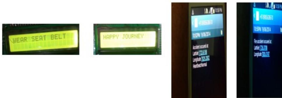
**Fig:** Photographs of LCD display indications and accident occurred, location and heart beat status messages send to mobile phones
